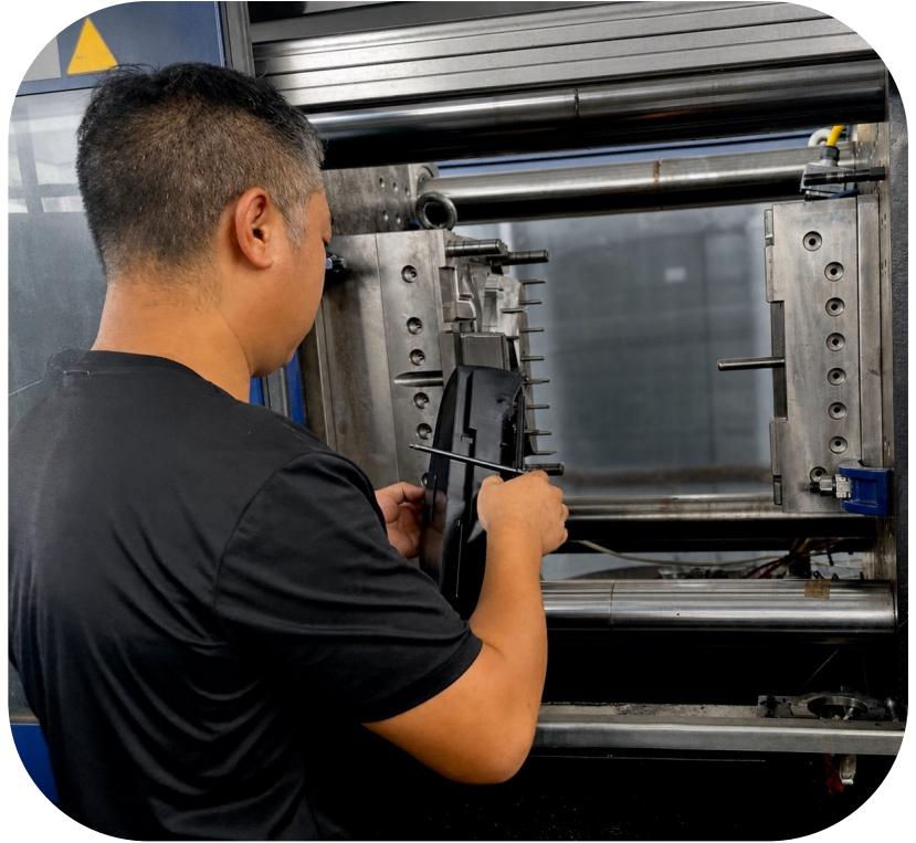
Trial Molding and Tool Adjustment
